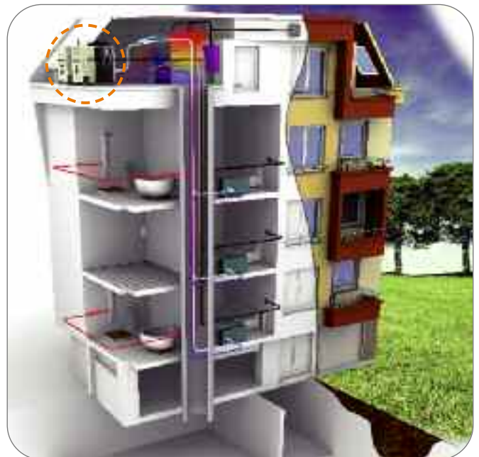
Example of GAHP-AR application in winter and summer operation for radiant panels, fan coils, indirect production of DHW.
