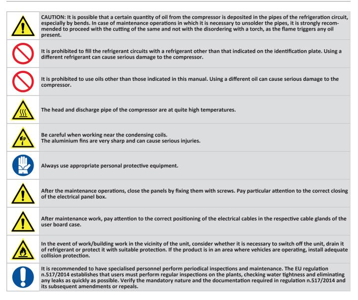
Plan all maintenance activities necessary for the safety of the unit. The following are the recommended (R), and mandatory (M), activities for correct operation of the unit. The mandatory activities must be carried out by an authorised customer service which issues a corresponding certificate. Failure to comply with these activities will entail forfeiture of the warranty and could considerably shorten the service life of your product.
