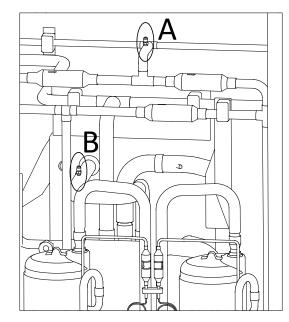
• flush the circuit by introducing nitrogen and bringing the pressure up to 4-5 bar. Expel nitrogen from the unit away from heat sources, igni-
