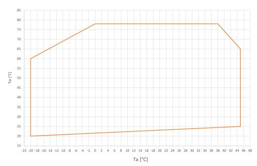
Tw = water temperature Ta = air temperature A = maximum Hz functionality has no effect
