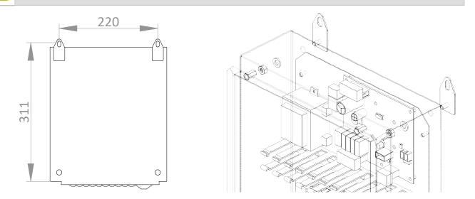
Connect the external kit to the heat pump via a cable suitable for modbus communication (cable not supplied, type to be used 3x0.5 mm<sup>2</sup> twisted and shielded). See the correspondence between the terminals of the user card and those of the kit in the table below:
