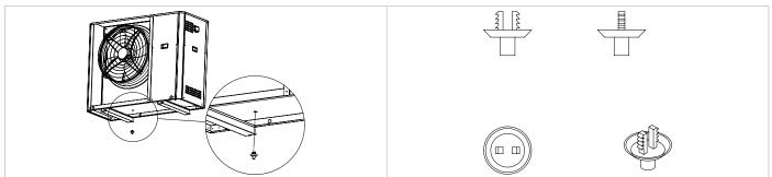
FOR HEAT PUMP UNITS, IN PARTICULARLY COLD CLIMATES, WE RECOMMEND THE INSTALLATION OF THE KA ACCESSORY, WHICH PREVENTS THE FORMATION OF ICE ON THE BASE FRAME.
