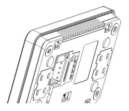
Drill holes in the wall and using screws (max.  $\emptyset$  3 mm) fix the installation frame in the selected place on the wall, maintaining its proper position (UP). The spacing of holes can be determined by placing the frame on the wall. Next fix the panel to the installation frame using latches.
