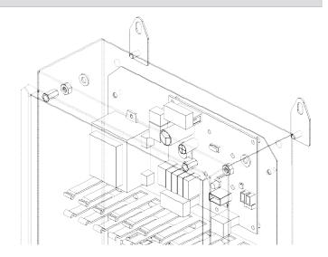
Connect the external kit to the heat pump via a cable suitable for modbus communication (cable not supplied, type to be used 3x0.5 mm² twisted and shielded). See the correspondence between the terminals of the user card and those of the kit in the table below:
