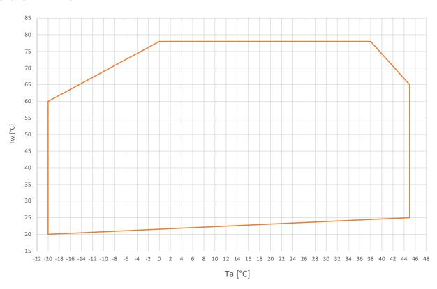
Tw = water temperature Ta = air temperature A = maximum Hz functionality has no effect
