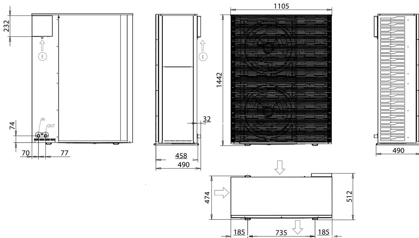
**5.7 POSITIONING OF CENTRE OF GRAVITY AND VIBRATION DAMPERS**
