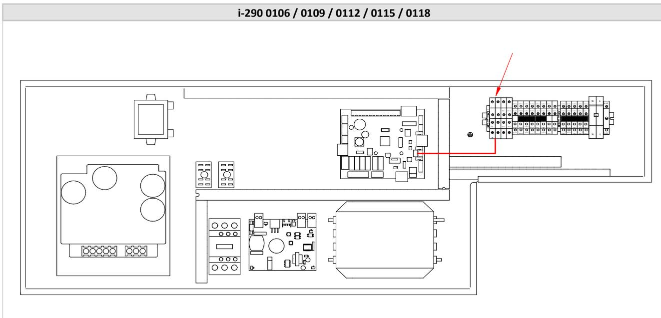
4. Connect the external kit to the heat pump via a cable suitable for modbus communication (cable not supplied, type to be used 3x0.5 mm<sup>2</sup>). See the correspondence between the machine terminals and those of the kit in the table below:
