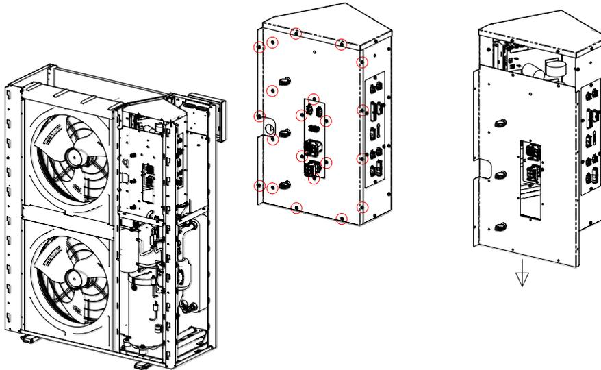
1. After removing the grilles, cover, side panels and angle brackets (as described in Chapter 5.7), unscrew the highlighted screws holding the cover of the electrical panel with a cross screwdriver.
