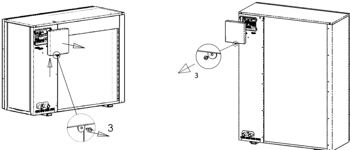
1. Unscrew screw M4 (number 3) using a cross screwdriver.
