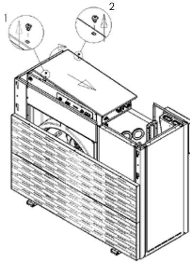
1. After removing the upper grille and cover (as described in Chapter 5.7), unscrew the screws holding the cover in place with a cross screwdriver (number 1, 2).
