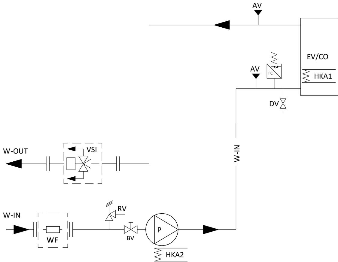
HYDRONIC CIRCUIT SINGLE PUMP VERSION (WITH OPTIONAL TANK)
