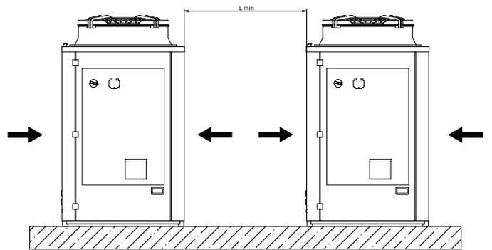
Covering with canopies or placing near plants or walls should be avoided to prevent air recirculation.
