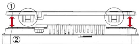
Disconnect the installation frame (1) from the back of room thermostat housing (2). The frame is attached to the panel housing with latches. Use a flat screwdriver to detach the frame.
