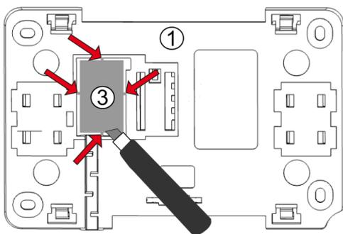
Using sharp tool cut out holes in four places of the cover (3) for the screw terminals.
