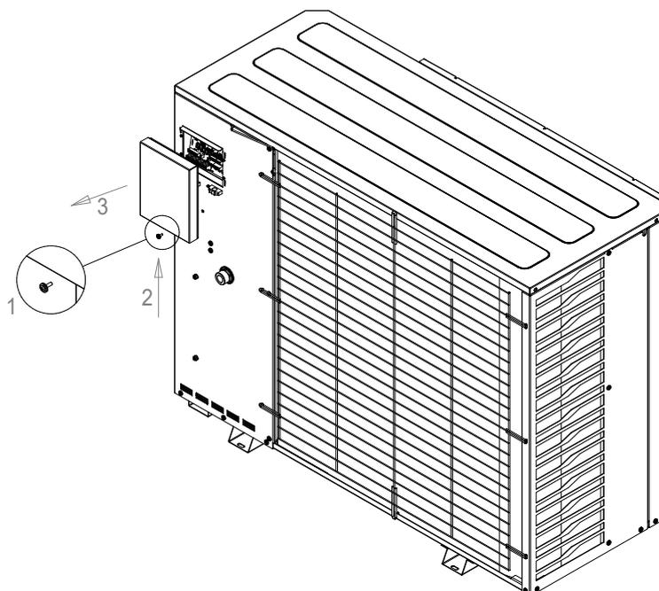
1. Unscrew the M4 screw (number 1) using a crosshead screwdriver.
