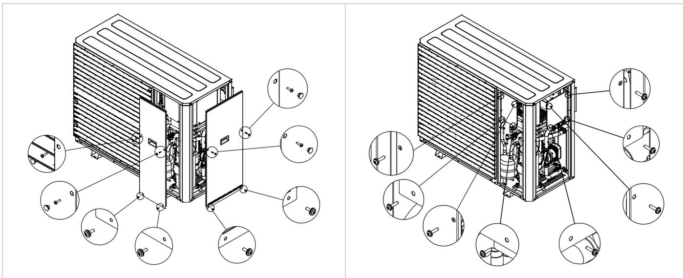
1. Remove the two access panels to the component compartment by unscrewing the screws as shown in figure 1.
