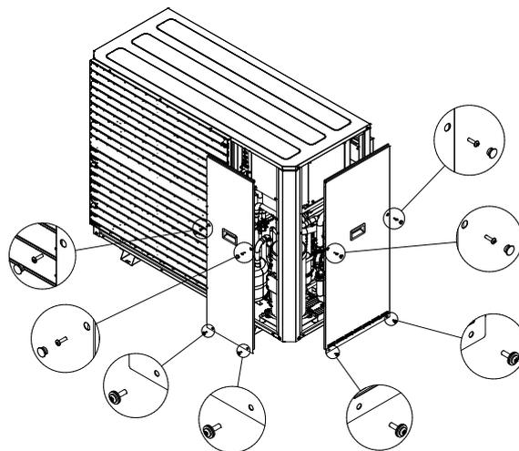
Remove the two access panels to the component compartment by unscrewing the screws as shown in Figure 1.
