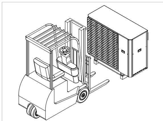
Lifting through forklift truck.
