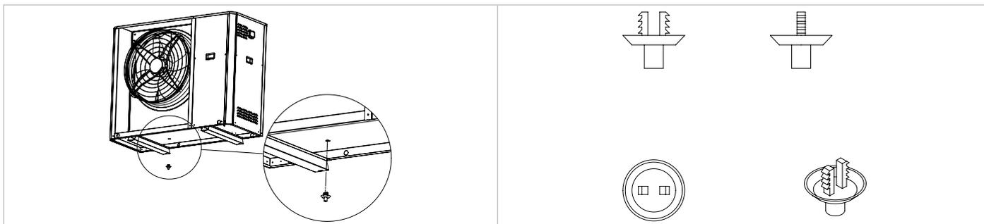
**FOR HEAT PUMP UNITS, IN PARTICULARLY COLD CLIMATES, WE RECOMMEND THE INSTALLATION OF THE KA ACCESSORY, WHICH PREVENTS THE FORMATION OF ICE ON THE BASE FRAME.**
