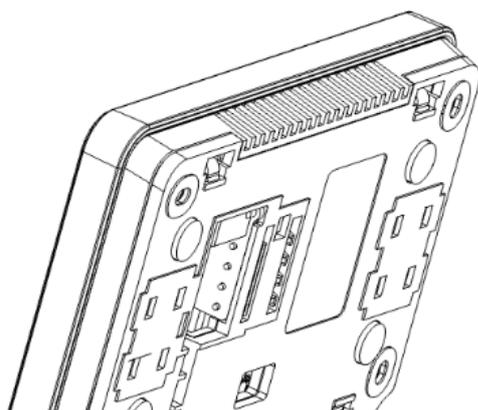
Drill holes in the wall and using screws (max. Ø 3 mm) fix the installation frame in the selected place on the wall, maintaining its proper position (UP). The spacing of holes can be determined by placing the frame on the wall. Next fix the panel to the installation frame using latches.
