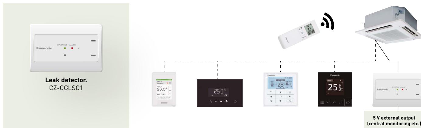
The alarm triggered by the leak detector will also be transmitted and displayed on any connected centralised controller.
