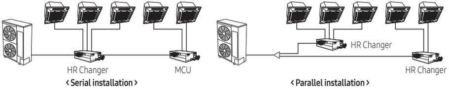
If the capacity of the indoor unit is under 5.6kW, don't use Y-connector.
