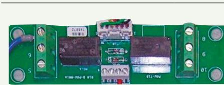
**T10 interface PCB with digital and relay connections.**
