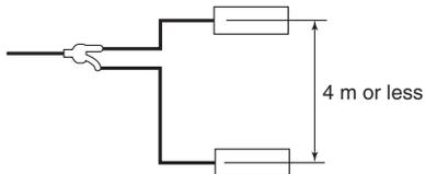
If height difference between indoor units after the final branch cannot be less than 4 m, divide the height difference between upper and lower units (2 to 1).
