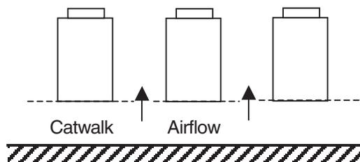
As shown in the diagram at the left, obtain  $L_U$  from the formula below by considering airflow from the bottom of the unit. However, if  $L_W \leq U_H + H_U$ ,  $L_U$  is the same as for concrete pads.
