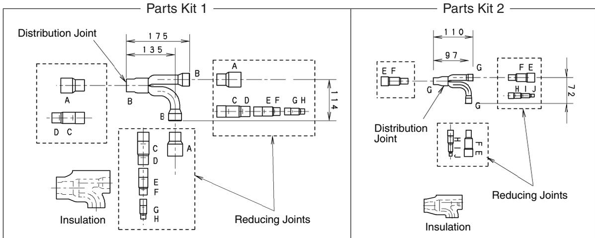
• Size of connection point on each part (Shown are inside diameters of tubing) (mm)
