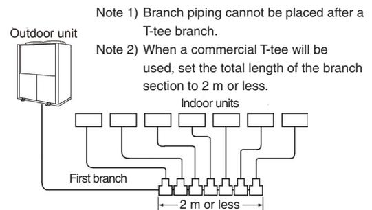
Note 1) Branch piping cannot be placed after a T-tee branch.
