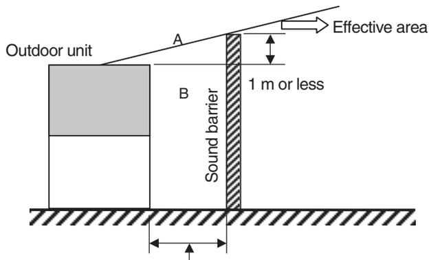
As close as possible (while maintaining minimum clearances required for intake, exhaust and servicing of each unit)
