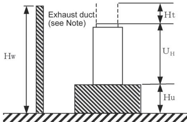
Note: When an air exhaust duct is used, take steps to prevent engine exhaust gas from entering the heat exchanger, such as extending the exhaust pipe to the same height as the air exhaust duct.
