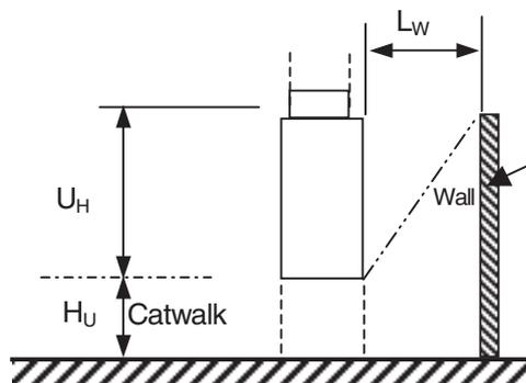
In the diagram at the left, if  $L_W \leq U_H + H_U$ , airflow to the catwalk is obstructed. Airflow from the wall side should be assumed to be zero.
