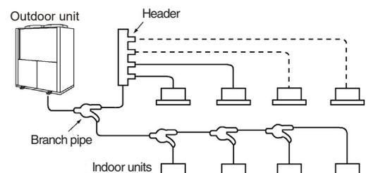
Note) All header piping openings are closed when shipping. Perform piping during expansion.
