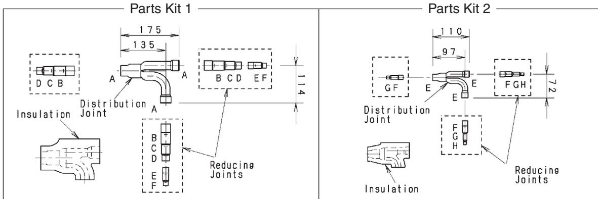
• Size of connection point on each part (Shown are inside diameters of tubing)
