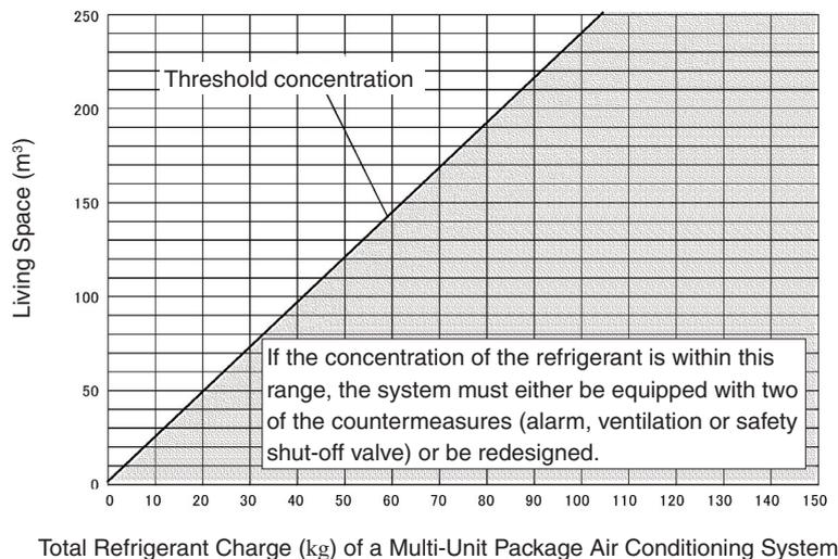
**Fig. 1 Permissible Refrigerant Charge for Specific Systems and their Required Countermeasures (R410A Refrigerant)**
