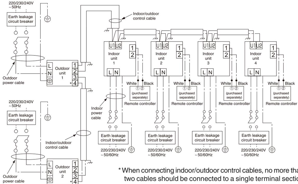
\* When connecting indoor/outdoor control cables, no more than two cables should be connected to a single terminal section on the terminal board. If you need to connect a third or fourth cable, connect the cables to 3 and 4 on the terminal board.
