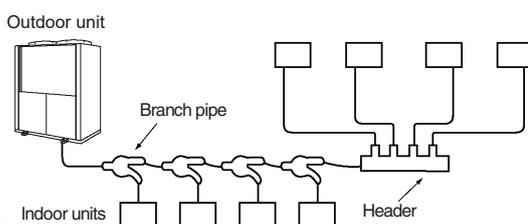
Note) Branch piping cannot be placed after a header branch.
