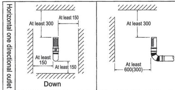
Figure 9 (Separation distance around the exhaust top)
