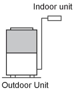
Refrigerant piping length: Over 90m (equivalent length)
