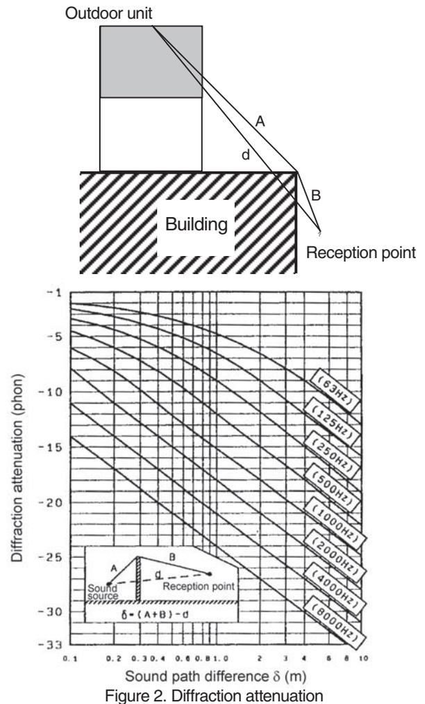
Figure 2. Diffraction attenuation
