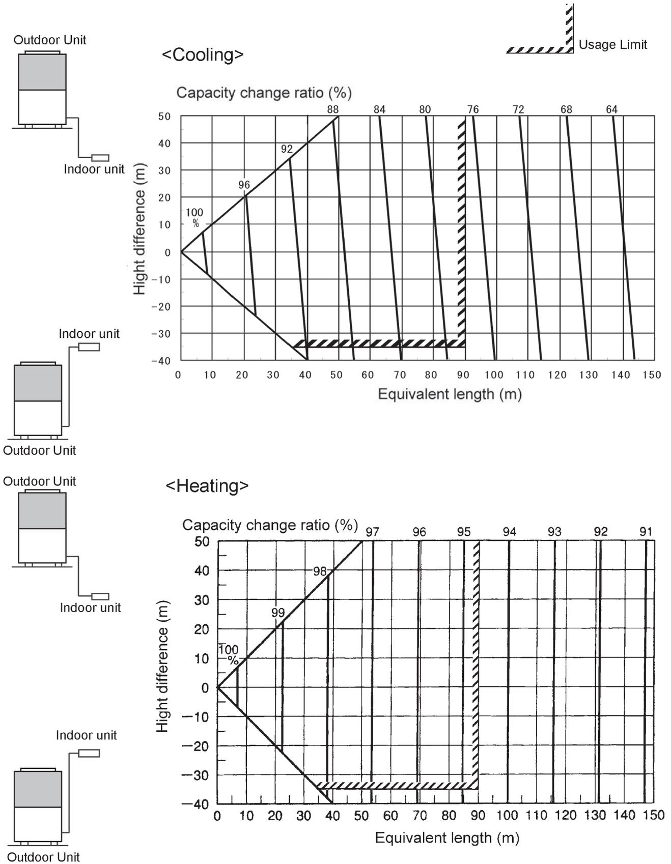
Refrigerant piping length: Over 90m (equivalent length)
