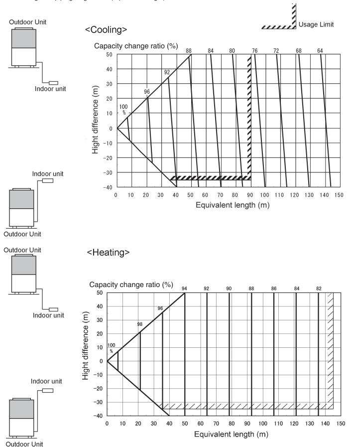
Refrigerant piping length: Over 90m (equivalent length)
