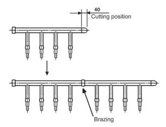
• For the cutting positions of the pipes, refer to the following figure.
