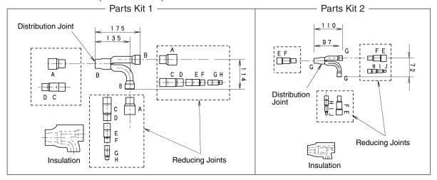
Size of connection point on each part (Shown are inside diameters of tubing)
