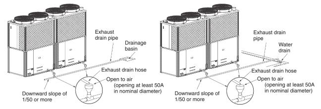
Fig. 12 Draining the exhaust into a drainage basin
